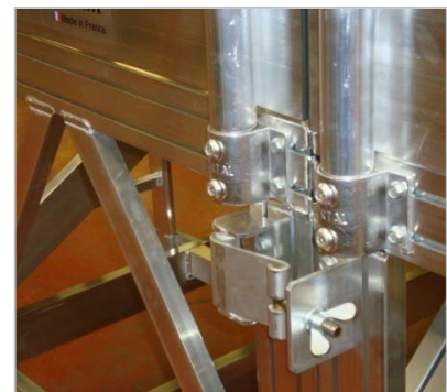
Quick assembly system of the 2 platform parts
