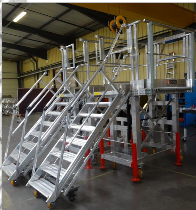
Rack system which allows the height adjustment of the platform
