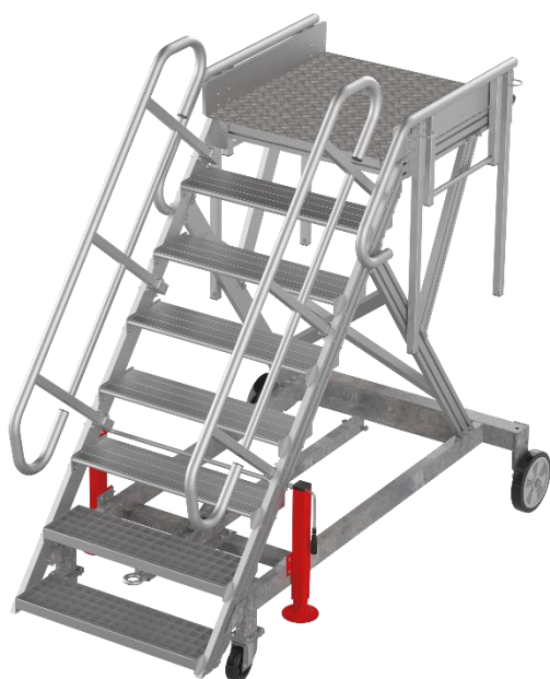
8-step stepladder – standard bearing – sliding guardrail – ramp with handrail and intermediary rail – anti-slip ribbed aluminum steps depth 261 mm Capacity of load 1 people + tools = 165 kg.
