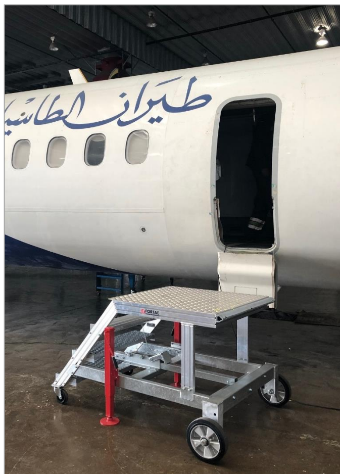
8-step stepladder – standard bearing – sliding guardrail – ramp with handrail and intermediary rail – anti-slip ribbed aluminum steps depth 261 mm Capacity of load 1 people + tools = 165 kg.
