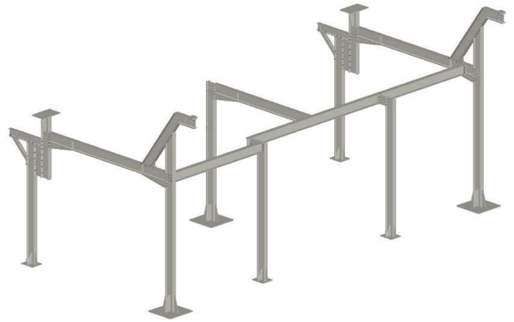
3D view steel support frame
