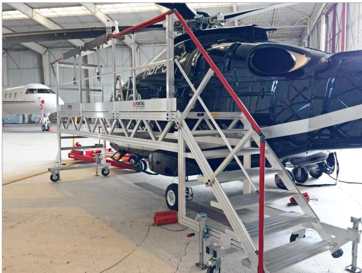
Platform equipped with 3 removable aluminum toolholders shelves.
