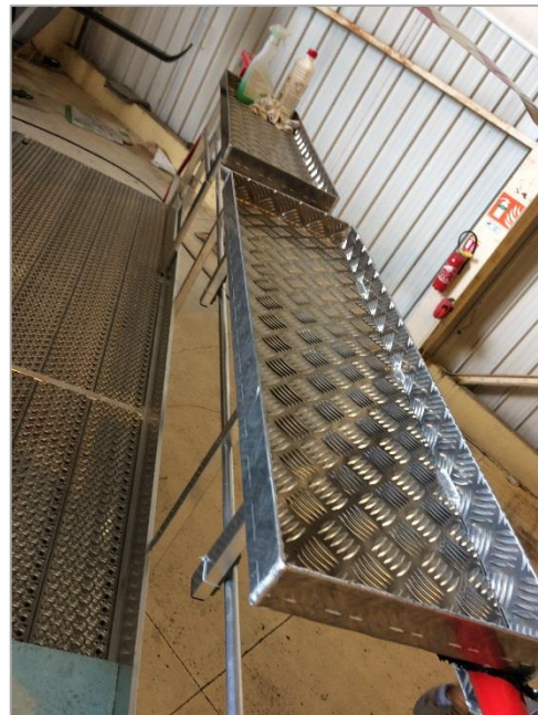
Platform equipped with 3 removable aluminum toolholders shelves.
