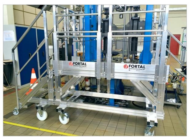
Raw extruded aluminum 100x30 mm platforms main structure, composed of:
