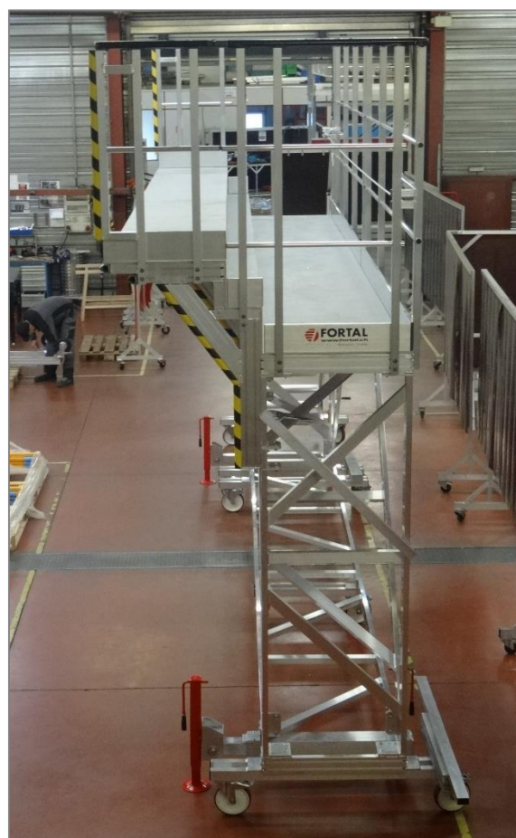
Platform 3 000 x 1 100 mm 350mm overhang with caoutchouc protection on plane side
