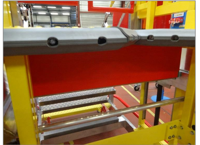
Foldaway rear step: risers red and green lacquered (visual identification during the climb/descent) Grating step yellow lacquered
