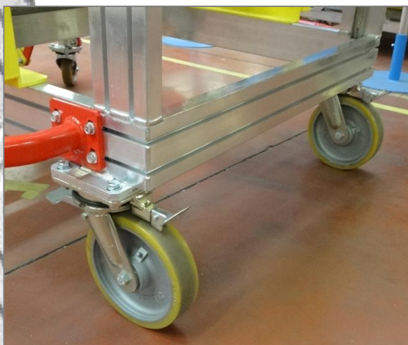
Swivel wheels with brakes 4 x 90° at the rear for easy moving
