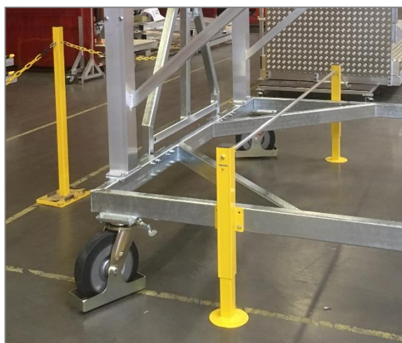
Platform moving with 4 swivel wheels without brakes with foot guards Ø 300 mm Immobilization by 2 pairs of twin outriggers
