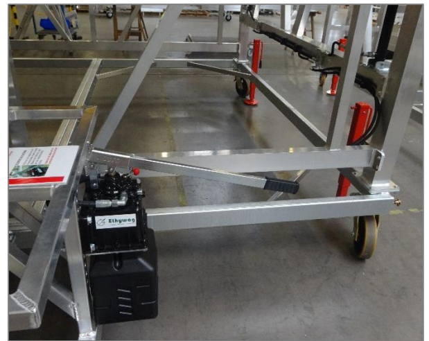
Working platform adjustable in height by hydraulic hand pump
