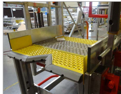
Retractable step on the rear side of the platform – Manually operated. Shockproof protection.
