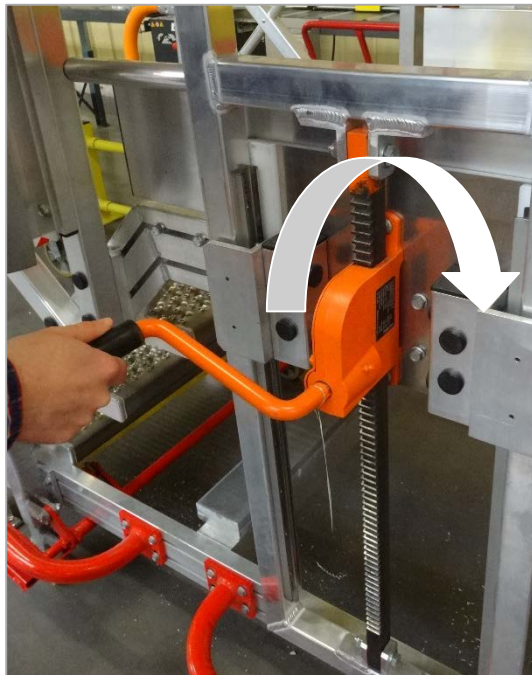
Side guardrail sliding vertically by rack system
