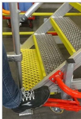
Side guardrail sliding vertically by rack system
