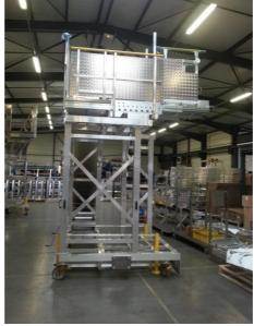
Platform mounted on rail, width 738 mm – adjustable in 2 directions :
