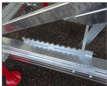
Mechanical locking system table in position
