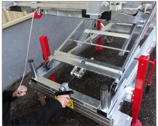
Height adjustable by only one person with crank – release of security by pulling a handful
