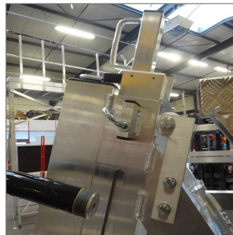
View of the stepladder deployment mechanism equipped with locking system by latch with spring
