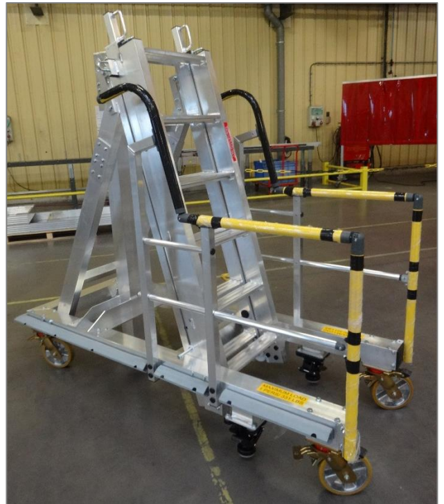
Anti-shock rubber protection on lower frame sides
