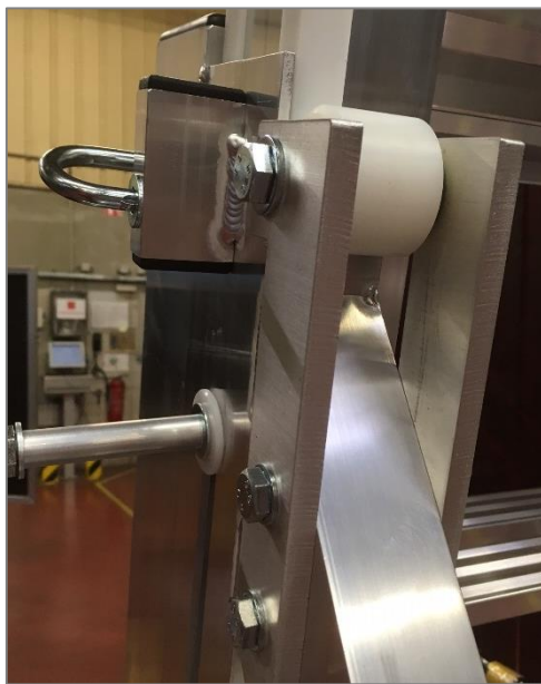
View of the stepladder deployment mechanism equipped with locking system by latch with spring
