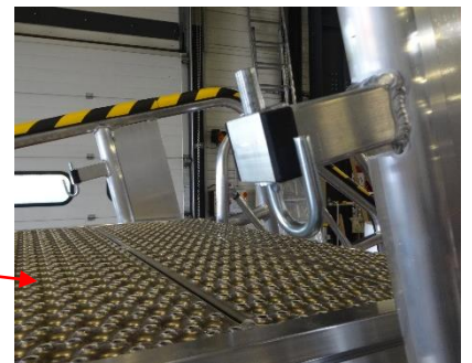
Grating platform coating Size: 770 x 700 mm View on guardrails locking system
