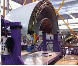
Realization of a mobile gateway with 4 subassemblies that, once juxtaposed, offer a confortable working area and allows staff to work on the engine covers in complete safety.
