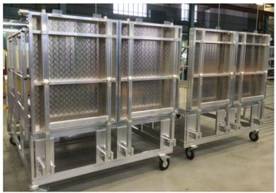
Once folded, with folded down trays, the subassemblies allow to save appreciable space when the gateway is not used.
